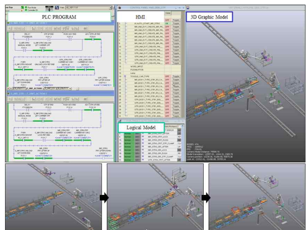
Figure 12. PLC simulation environment of SQ & SIL
