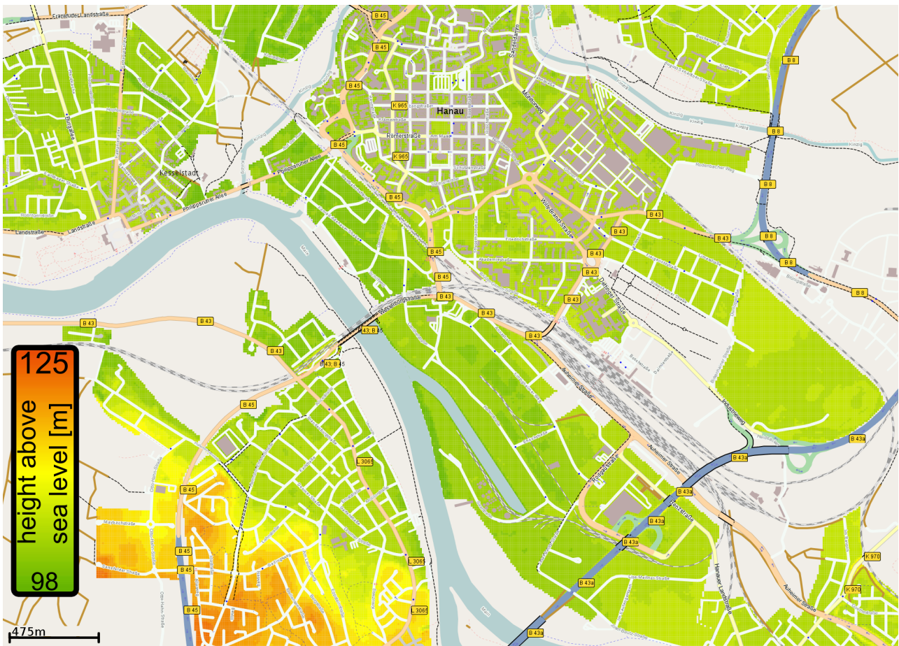
Figure 3: Extract of simulated map area, representing Hanau am Main (89,000 inhabitants), Germany with the corresponding extract of the DTM. Total length of roads: 548km, number of nodes in simulation graph: 4,201, number of edges: 5,758.
